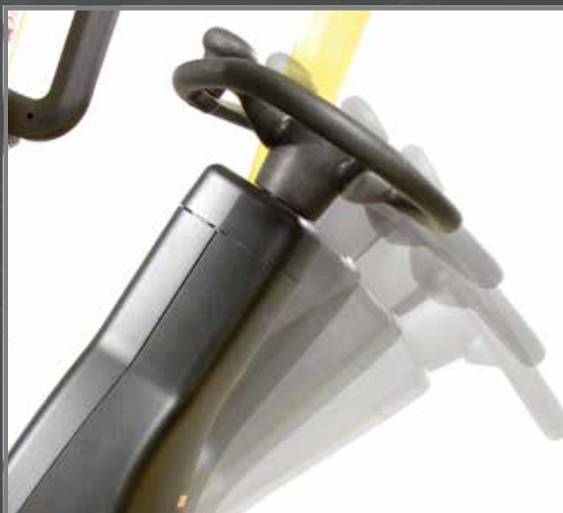
Infinitely adjustable tilt steer column
