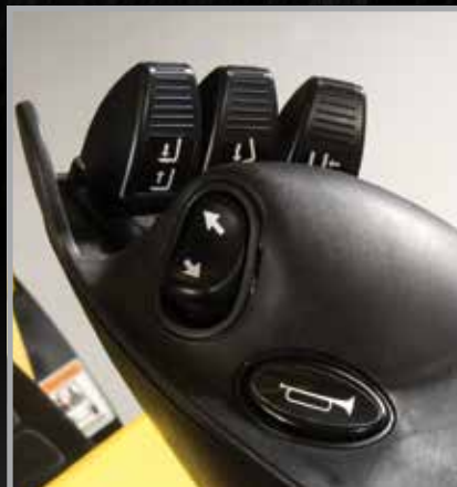
TouchPoint mini-levers with seatside direction control
