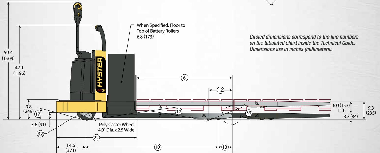
*Circled dimensions correspond to the line numbers on the tabulated chart inside the Technical Guide. Dimensions are in inches (millimeters).*
