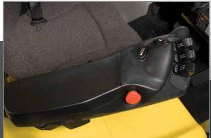
Electro-hydraulic controls with TouchPoint mini-levers
