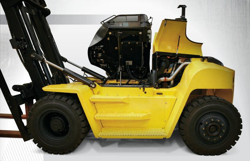
All engine, transmission and other service check points are conveniently situated for quick maintenance. The daily service checks can be completed in less than 10 minutes and do not require the cab to be raised. The hardest decision you will have to make as an owner of an H190-360HD<sub>2</sub> series truck is electric or manual tilt.
