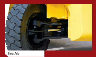
The Hyster hydrostatic steer axle is as tough as they come. It's maintenance free and that's not easy with the beating it takes. Its durable spindles are supported by pre-lubricated tapered roller bearings which resist shock and wear. Periodic adjustment is eliminated by its fixed length tie rods. Adjustable steer axle stops can be adjusted to extend tire wear, when extreme maneuverability isn't required, to dramatically improve steer tire life.
