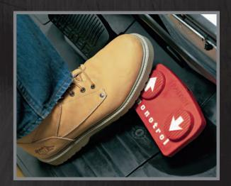
Inching and braking are not the same. On the H190-360HD<sub>2</sub> lift truck series you have two pedals, one located on either side of the steering column. The left-hand side pedal provides you braking and inching capabilities by partially disengaging transmission clutch packs. Fully depressing this pedal engages the brakes. The brake pedal is on the right-hand side of the column.
