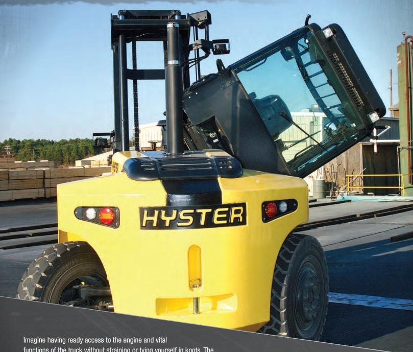
functions of the truck without straining or tying yourself in knots. The answer is the side tilting ComforCab II of the Hyster® H190-360HD<sub>2</sub>. The cab, mounted on 4 rubber isolators pivots over to the right-side of the truck, giving you complete access to all the major components.
