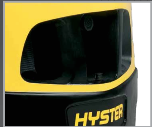
Counterweight tunnel design improves airflow
