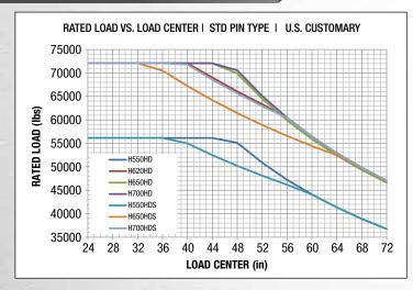
Model H550HDS: 55,000 lbs. at 36" (24,948 kg at 914 mm) load center Model H650HDS: 65,000 lbs. at 36" (29,484 kg at 914 mm) load center Model H700HDS: 70,000 lbs. at 36" (31,752 kg at 914 mm) load center Model H550HD: 55,000 lbs. at 48" (24,948 kg at 1219 mm) load center Model H620HD: 62,000 lbs. at 48" (28,123 kg at 1219 mm) load center Model H650HD: 65,000 lbs. at 48" (29,484 kg at 1219 mm) load center Model H700HD: 70,000 lbs. at 48" (31,752 kg at 1219 mm) load center
