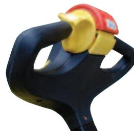
◀ The standard creep speed feature greatly increases maneuverability by allowing the W40Z to operate with the handle in the full upright position. With the Freighter’s Special option, the steer handle is kept away from the side of the trailer during pin-wheeling.
