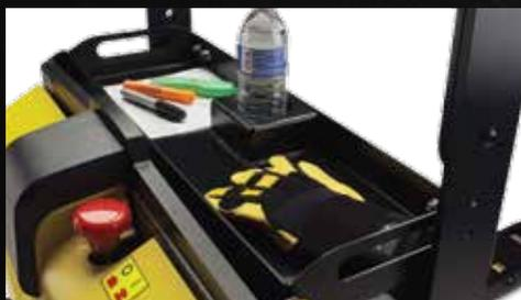
*The W45Z<sup>HD</sup> with factory installed batteries includes an operator convenience tray with large storage area for stowing clipboards, pens, pencils and other items. Units equipped with a 9" battery box have several convenience tray options. (9" battery box option shown)*
