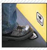
Mounted in the floor plate, the high speed or "rabbit" speed switch gives the T5-7Z<sup>AC</sup> Tow Tractor series' excellent travel speeds. So whether you're towing one or more carts your operators spend less time traveling, for enhanced productivity and a better bottom line.
