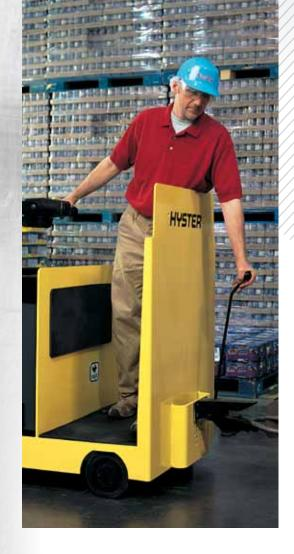
Spacious operator's compartment is 20.8" deep and 32.0" wide. It comes equipped with a forward bulk-head, operator's back pad, and a shock absorbent, removable 1.0" thick floor mat affording ample cushioning. It also reduces the effects of vibration and standing stresses, while enhancing operator stability over uneven surfaces. Best of all, with a 9.8" step height, entry and exit is easy.
