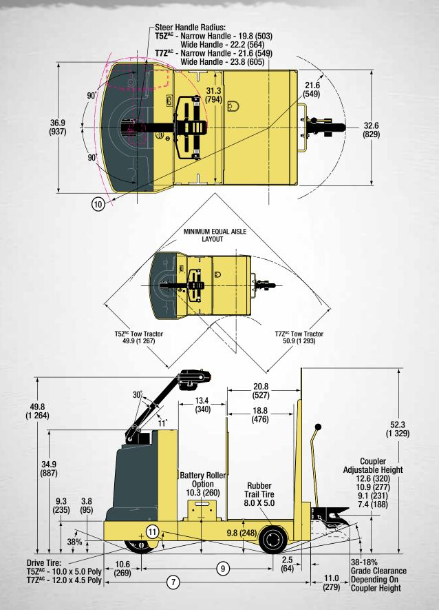
Circled dimensions correspond to the line numbers on the tabulated charts on Page 6 and 7. Dimensions are in inches (millimeters).
