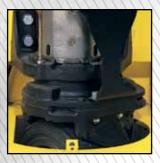
Sealed and bathed in oil, the Master Drive Unit (MDU) bearings provide quiet, smooth, low effort control of the T5-7Z<sup>AC</sup> Tow Tractor series. Its muscular Master Drive Unit has an integrated pinon gear with a splined coupling for ease of service.
